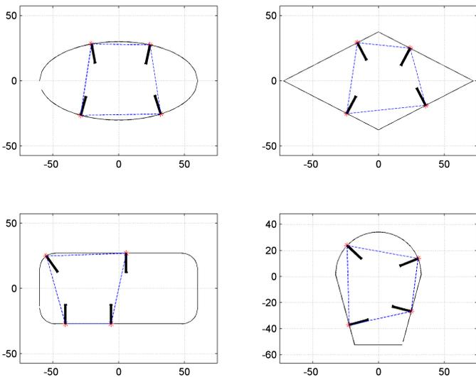
Fig. 5. Solution of a 4-finger common grasp ( $k = 150$ ).
