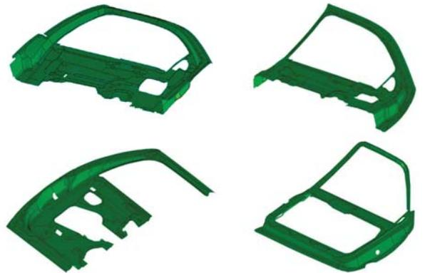
Fig. 5. CAD's of four sheet metal parts.
