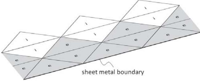
Fig. 3. The triangles of the mesh marked to be edge or inner triangles when  $m = 3$ .
