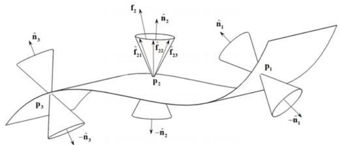
Fig. 2. Grasping of a sheet metal part.
