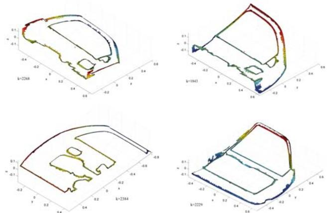
Fig. 6. Four boundary meshes of the sheet metals.
