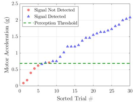
Fig. 3. Experimental results for the vibrotactile stimulation perception threshold in a canine subject. The trials were conducted in random order, but are displayed by order of amplitude.
