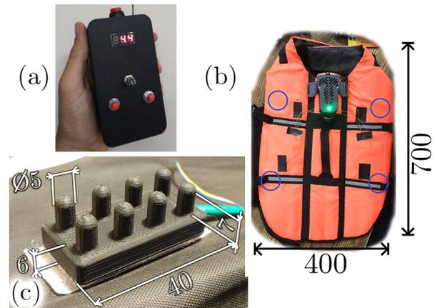
Fig. 1. (a) The transmitter has two buttons (red) at the bottom. The amplitude dial is in the center, and the amplitude is displayed on a screen (top). (b) The receiver vest has a receiving unit (black with green LED) that receives commands from the transmitter and activates embedded vibration motors (locations marked in blue circles). (c) The vibration motor housing has prongs that are intended to penetrate the fur and deliver the vibration to the skin. All dimensions are in mm.
