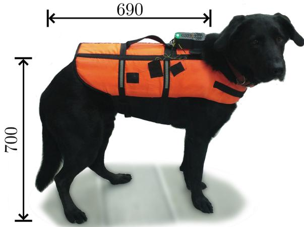
Fig. 2. The test subject wearing the vibrotactile vest. The receiving unit (black with green LED) receives the commands from the transmitter and activates embedded vibration motors. Basic body dimensions are shown in mm.
