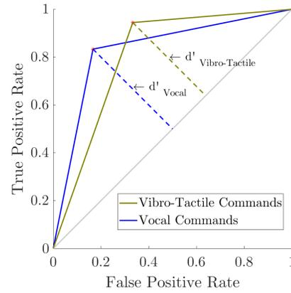
Fig. 4. The ROCs for the test subject’s response to vocal and vibrotactile commands, for 30 trials.
